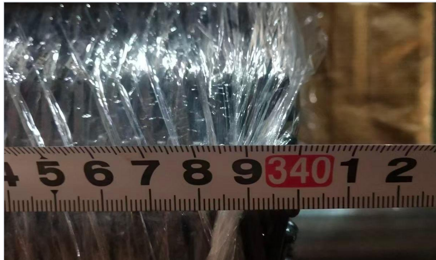
Width re-checked on the roll
