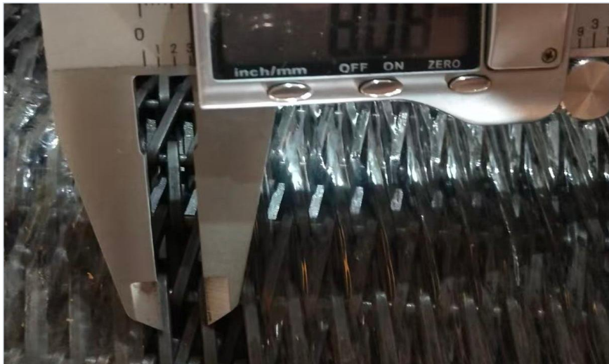
Spiral pitch re-checked after wrapping
