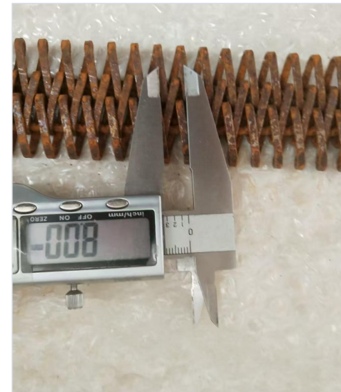
Spiral pitch measured on the sample
