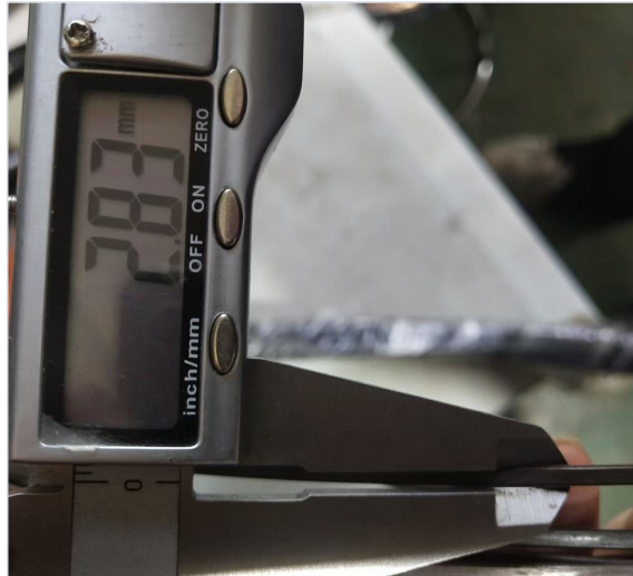
Flat wire measured
