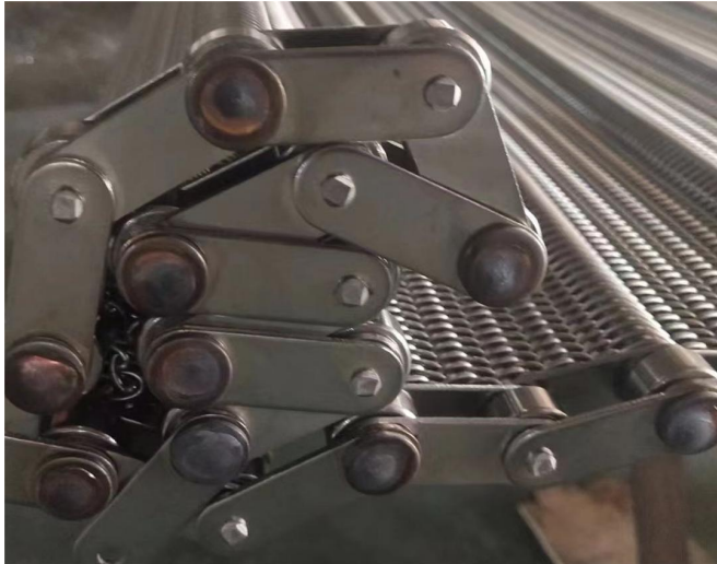
Exposed chain, rod and mesh connections
