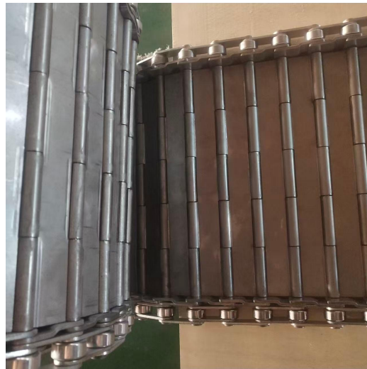
Plate surface and side-chain assembly
