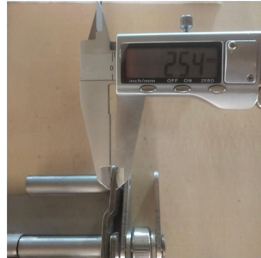
Side-guard thickness measurement
