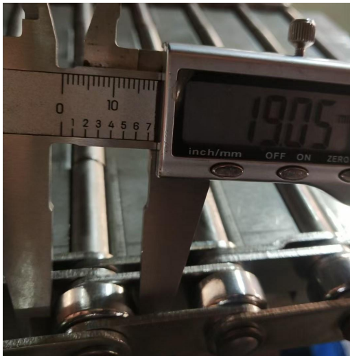
Roller measurement in the first-article records
