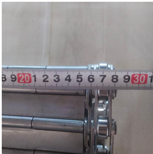
Overall-width check on the 282 mm variant
