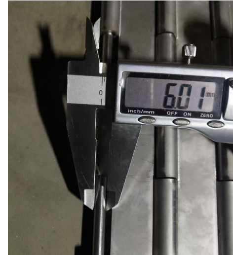
Cross-rod diameter measurement
