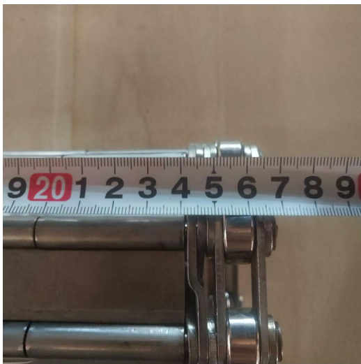
Overall-width check on the 257.2 mm variant
