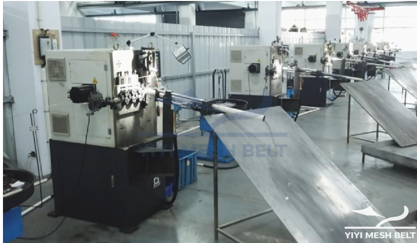
Spiral forming equipment
