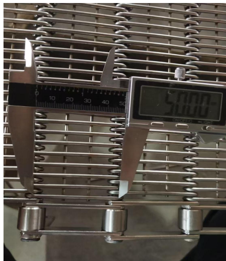
50 mm rod-pitch check on the other variant
