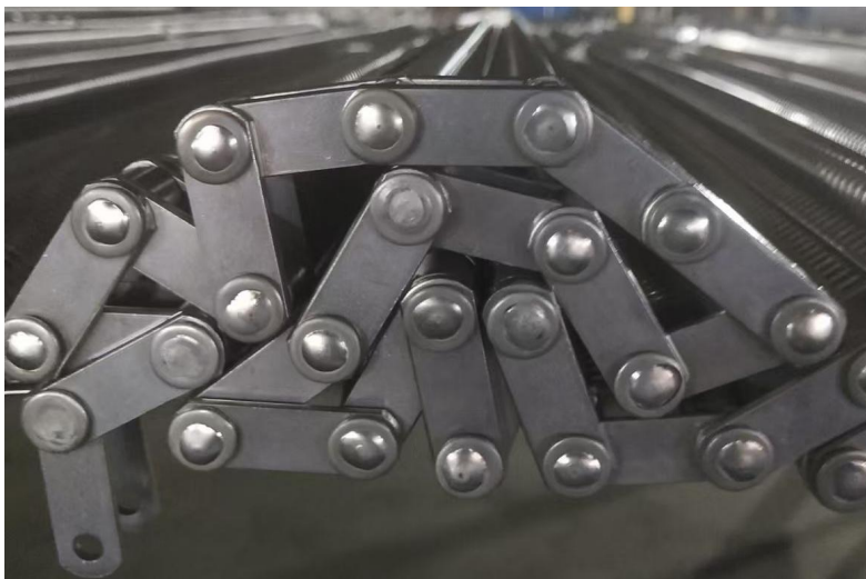
Assembled side chain and connecting rods
