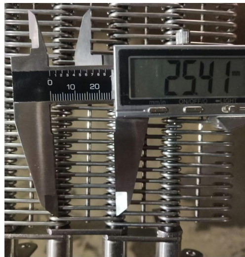
Rod-pitch measurement in the first-article photo set
