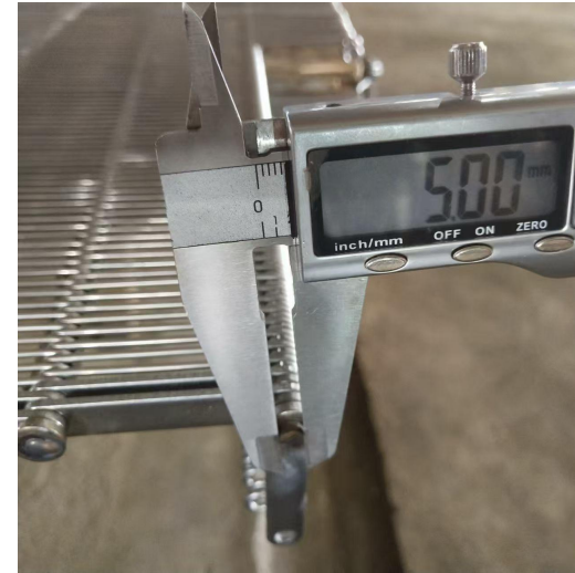
Cross-rod diameter measurement
