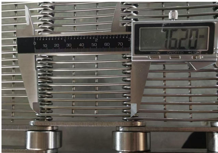
76.2 mm rod-pitch check on one variant
