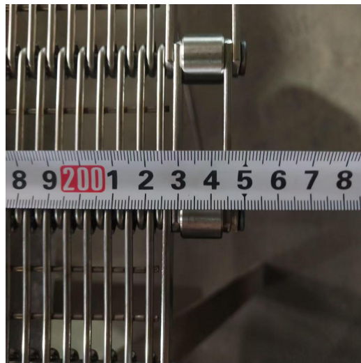
Overall-width measurement on the 2,052 mm variant
