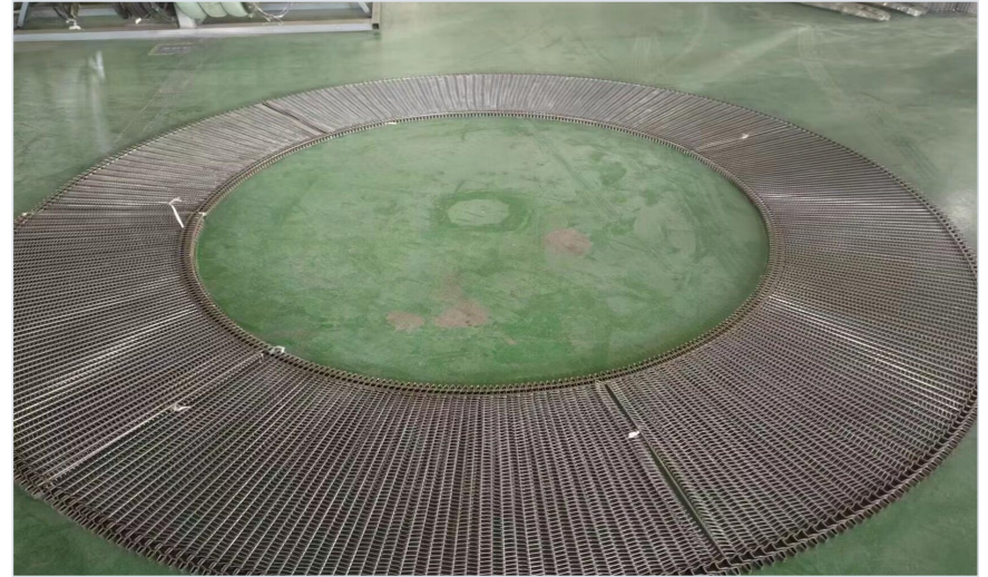
Belt laid out at the turning diameter (earlier order)
