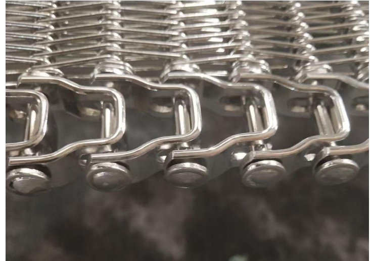
Washer-welded edge in the same order
