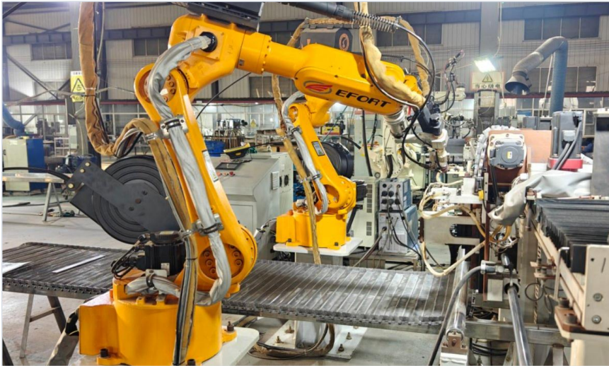
Robot welding cell
