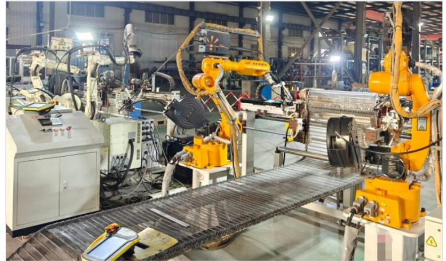
Robot welding line
