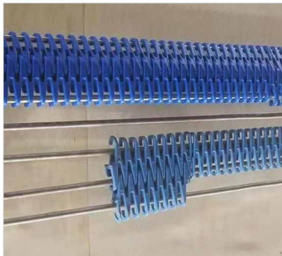
Thailand: replacement side driven belt
